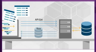
API exposing a lot more data than the client legitimately needs, relying on the client to do the filtering. Attacker goes directly to the API and has
