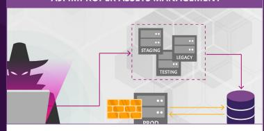
Attacker finds non-production versions of the API: such as staging, testing, beta or earlier versions - that are not as well protected, and uses those to launch the attack.
