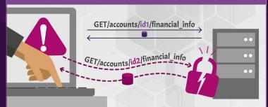
Attacker substitutes ID of their resource in API call with an ID of a resource belonging to another user. Lack of proper authorization checks allows access. This attack is also known as IDOR (Insecure Direct Object Reference).
